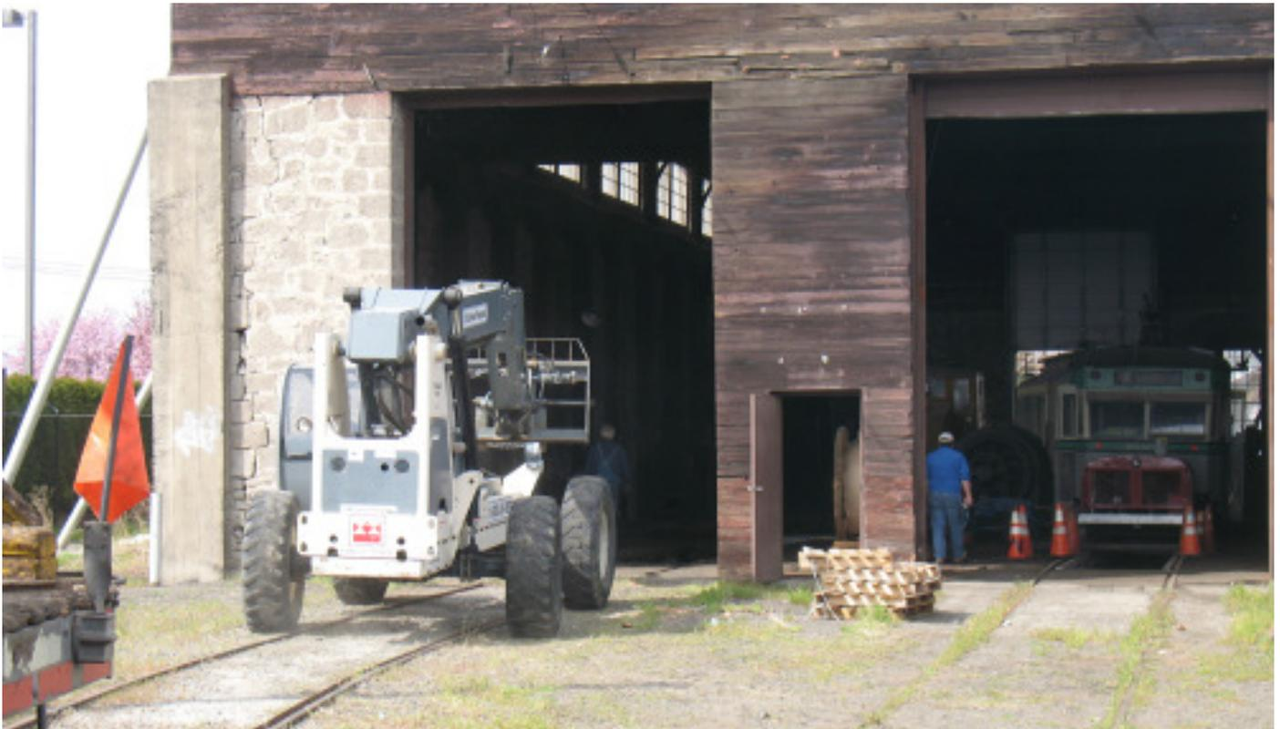
To help clean out the west wall of the carbarn the group rented an extendable boom forklift. The boom extension came in handy to reach items along the wall while keeping the weight off the wood floor. Scott Neel ran the lift while Rich Wilkens and others helped in slinging loads.
